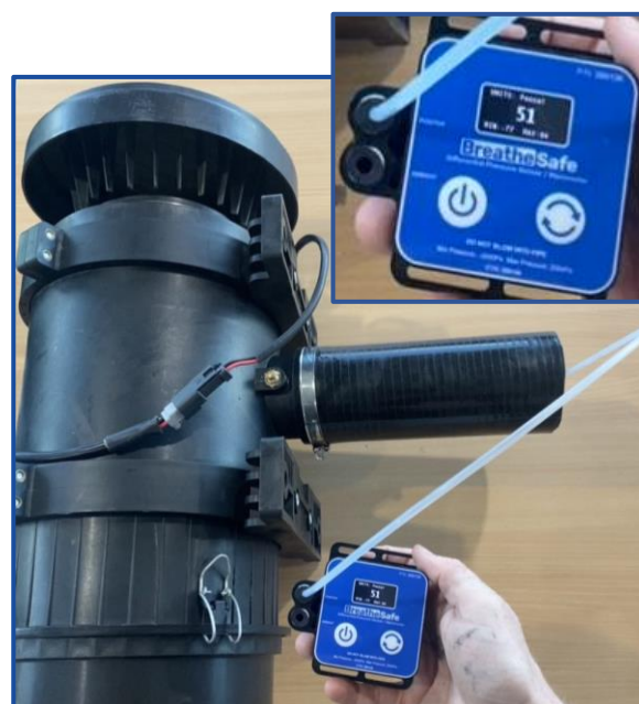
Figure 1: False positive pressure reading when blowing into open air
