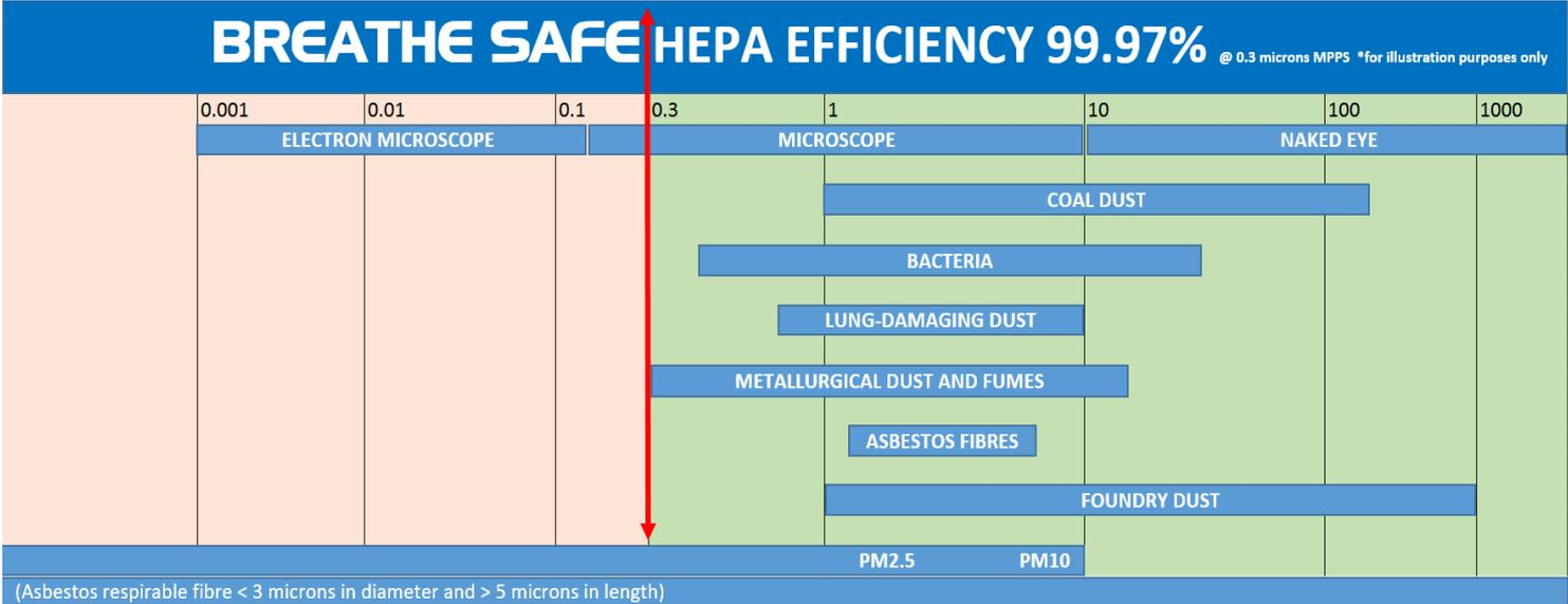
Table 3. HEPA filter media efficiency chart. (Asbestos respirable fibre < 3 microns in diameter and > 5 microns in length).
