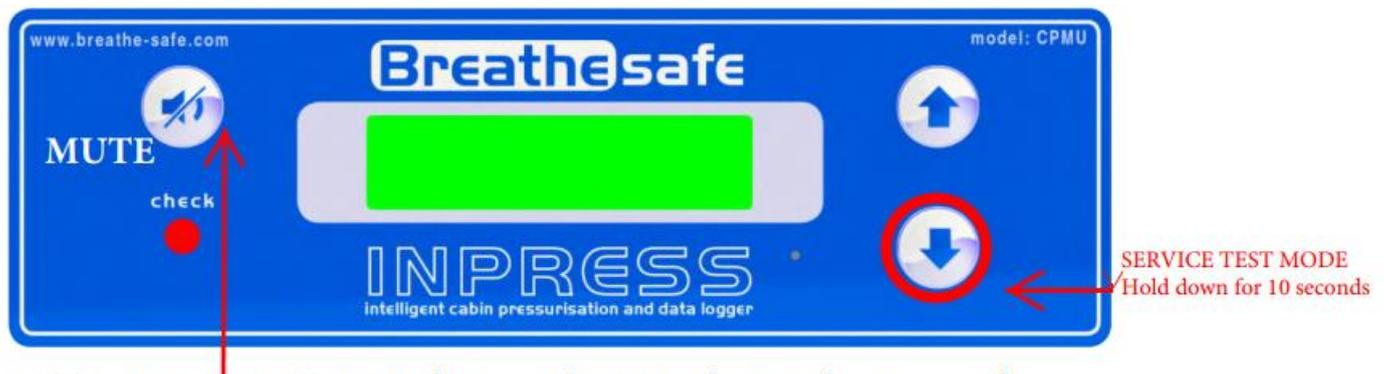
\*\* To exit Service Test Mode press the Mute button for 2 seconds
