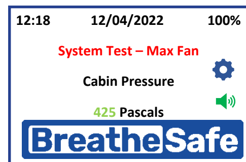
Record / Photograph the cabin pressure result (Max Fan Speed).
